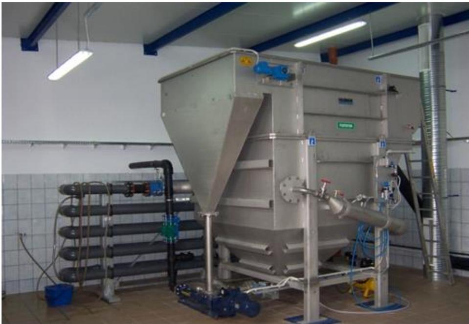
► HUBER Dissolved Air Flotation HDF for advanced (waste)water treatment with micro bubbles
